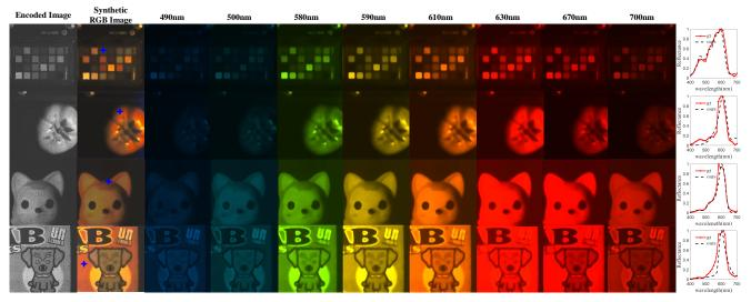
Figure 9. Experimental results of different scenes, the first column is the captured coded image, the second column is the synthetic RGB image with the recovered spectrum, the 3-10 th column is the recovered hyperspectral channels, the last row is the comparison between the recovered spectrum with the spectrum captured by a ASD spectrometer.
