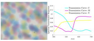
Figure 2. (a) Image of ink droplet distribution at micron level. (b) Spectral transmission response of CMY color printed film.
