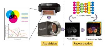
Figure 1. Overview of the proposed hyperspectral imaging system: with a consumer-level printer, a random color printed mask can be attached to the sensor of the camera to sample the hyperspectal images. Through randomly overlaying ink droplet, the spectral transmission response of different points is rendered high uncorrelated and faciliate the full spectrum recovery with details. A convolutional neural network is proposed to recover the hyperspectral images from the randomly coded images.
