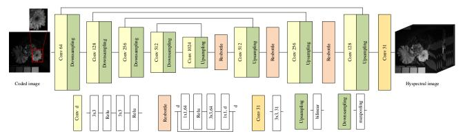
Figure 6. CNN-based network structure. The input an spectrally coded RGB images by our color printed mask, and the output is the predicted hyperspectral images of 31 channels. The multiscale network is composed of convolution layers, bilinear upsampling, maxpooling and Resbottle modules, which can exploit correlation among pixels over receptive fields of different scales with an elegantly amount of parameters.
