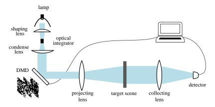
Fig. 5. The schematic diagram of CGI. Light source: high pressure Mercury lamp (Philips, 200w). DMD: Texas Instrument DLP ® Discovery  $^{TM}$ 4100, .7XGA. Scene: a transmissive film (34mm $\times$ 34mm). Detector: Thorlabs DET100 Silicon photodiode (integration time: 0.625ns).
